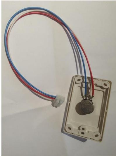
Figure 9. Rear of variable resistor showing terminals.
