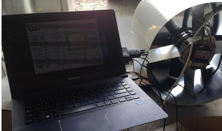
Figure 11. Motor controller programming.
