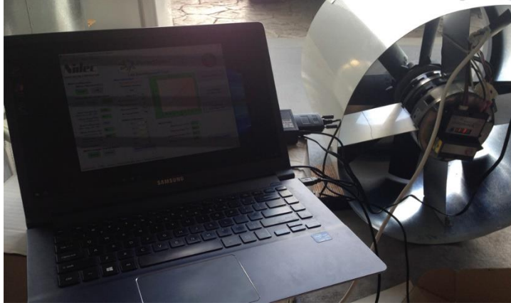
Figure 11. Motor controller programming.
