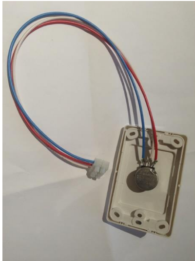
Figure 9. Rear of variable resistor showing terminals.
